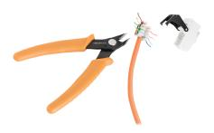
NIKOMAX NMC-222 is designed for precision cutting wires and other delicate electrical work. Pliers length of the cutting edge - 10 mm. Suitable for copper conductors and other soft metals to 1 mm (18AWG). Not suitable for steel.
