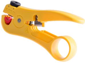
Tool NMC-350 is designed to remove the insulation and trimming with twisted pair. The presence of the wheel for fine adjustment of the depth of the knife moves allows you to make an accurate cut without damaging the insulation of the conductors under the outer shell. A distinctive feature of the NMC-350 is the presence of a spring-loaded cradle for a smooth and uniform course when scrolling around the cable. And the ergonomic design will provide even greater comfort when working.
